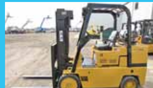
Cat TC100D Forklift, gas, 2WD, 10,000# lifting cap, 4,230 hours, inside cushion tire, propane, good strong unit, $9,850
