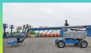
2008 Genie Z80/60 Articulating Boom Lift, 500# lift capacity, 80' platform height, 2,474 hours, $38,505
